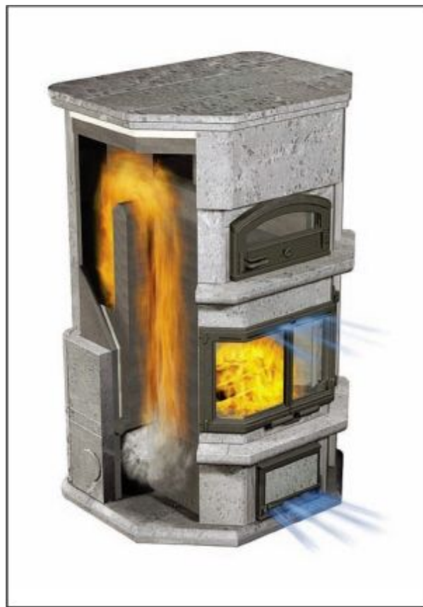
FIGURE 8.54. In a Finnish contraflow design, the exhaust travels up through a throat into a secondary combustion chamber then flows downward, typically on both sides of the heater. Then the smoke exits to a chimney connector at the base. In this cutaway photo, only one side can be seen. Photo courtesy of Tulikivi Corporation.
