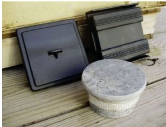
FIGURE 12.5. Some of the cleanout (soot) doors available. Both of the black doors are held into their frames by gravity. The soapstone plug fits by friction of the fiberglass rope inside a sawn-out circle. See figures 2.1 and 7.16 for square tile cleanout covers that are held in by clay mortar.
