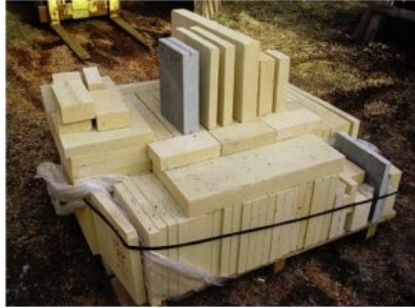
FIGURE 8.19. A partial pallet of heater materials. Standing on top is the soapstone and all the refractories used to build this chapter's project. From left to right: 23.8-inch soapstone; 11.4-inch refractory plate; 11.2-inch refractory plate; 21.2-inch refractory plate; 21.2-inch firebrick; and 2-inch firebrick. The thinner plates are 12 inches square while the 21.2-inch plate is 12 by 24 inches.
