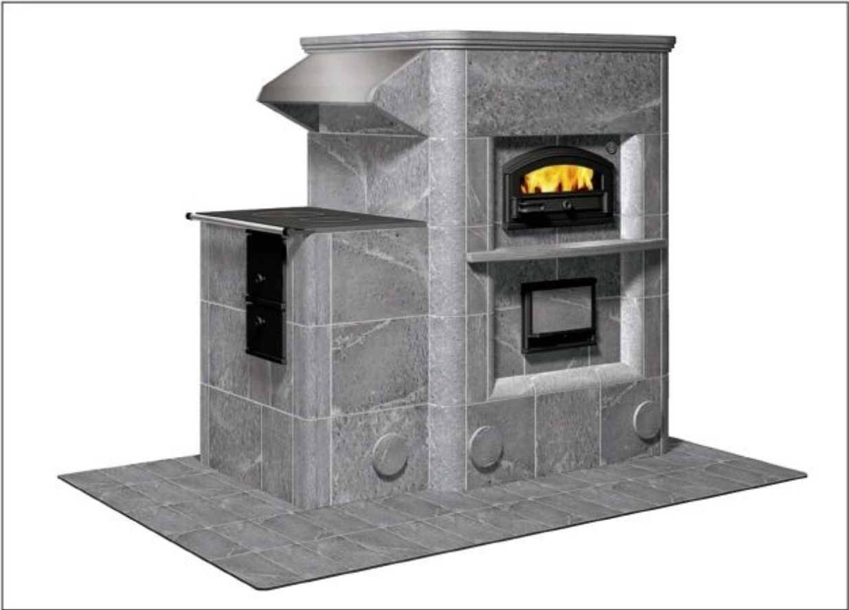
FIGURE 11.12. The baking chamber in this masonry heater is the primary firebox for warming the whole mass. A cookstove is added to the side of the bakeoven, turning this into a complete cooking complex. Photo courtesy of Tulikivi Corporation.
