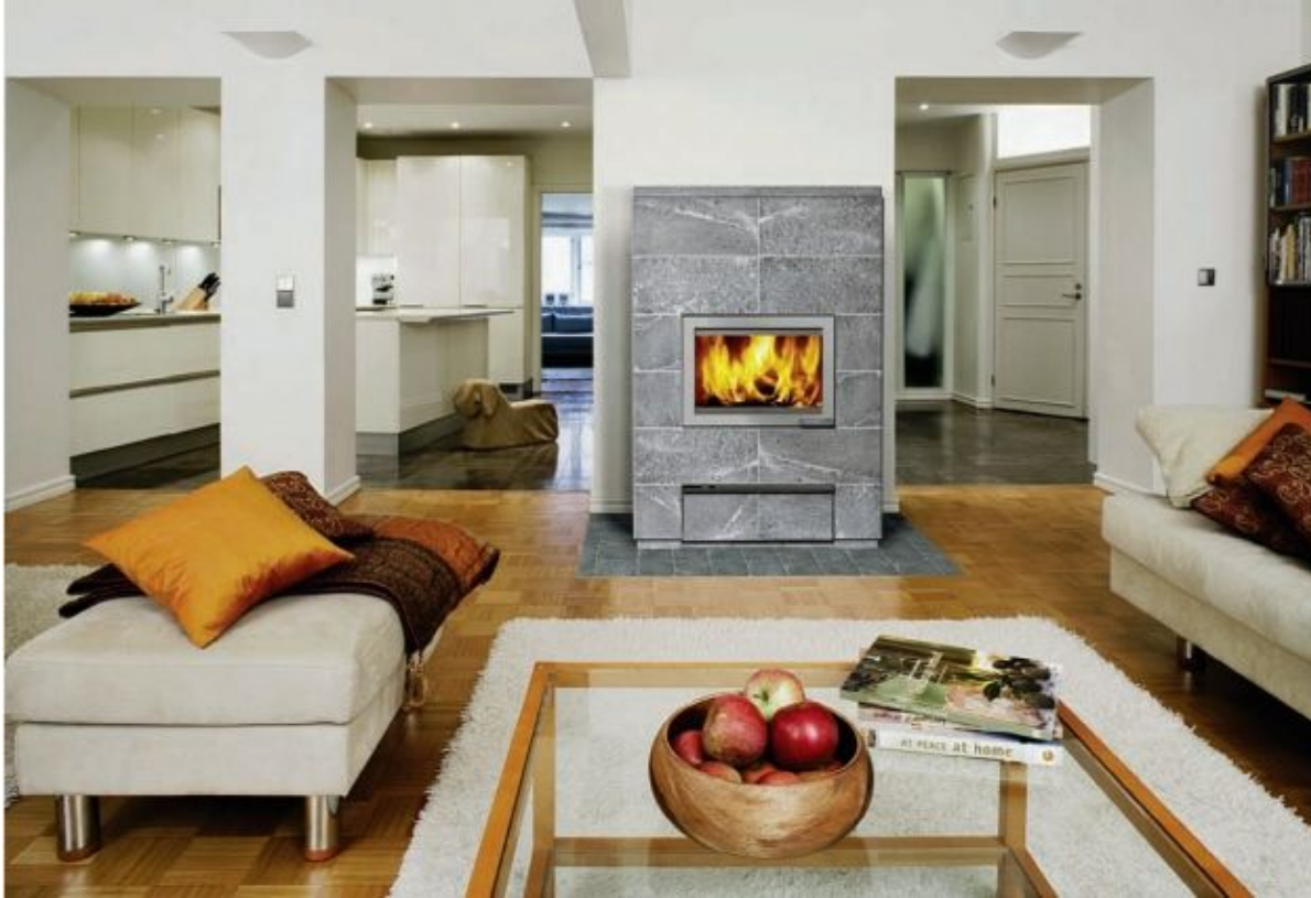
FIGURE 6.8. You might think the heater pictured here has no chimney, because the flue has been artfully hidden in the wall behind. This is one of Tulikivi's newest, more modern designs featuring a new firebox design (see chapter 8 ) and soot doors hidden inside the ash drawer access area below the firebox. This makes for clean, unbroken lines. Photo courtesy of Tulikivi Corporation.
