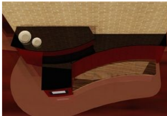
FIGURE 6.14. The plan view shows the unusual shapes possible in masonry heater design.
