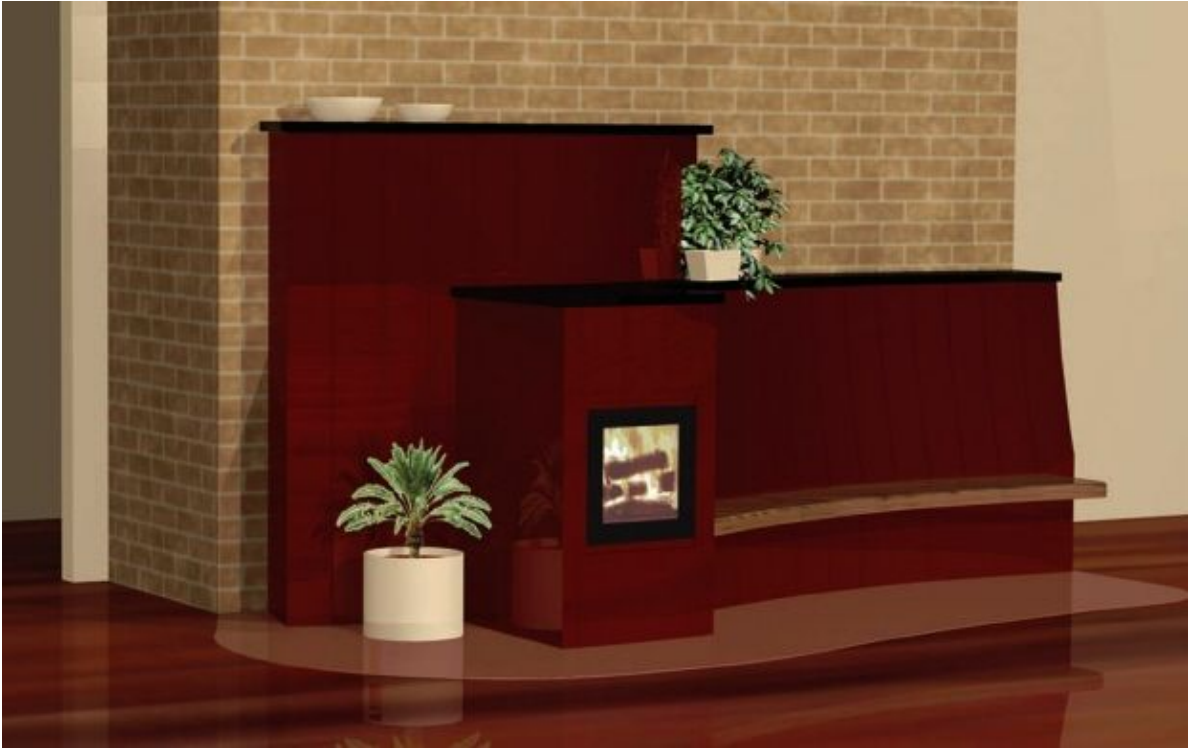
FIGURE 6.13. A one-of-a-kind masonry heater designed to fit a customer’s taste, decor, and living space. This concept has been approved, with slight modifications, by the client and will be constructed of structural tiles for a residence in southern Ohio.
