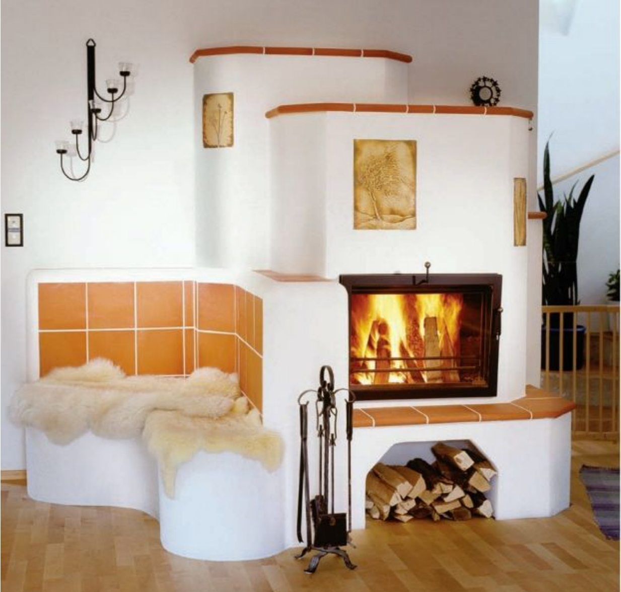
FIGURE 7.9. This stucco heater with tile trim features a heated “couch.” Notice the wood storage under the firebox and specialty picture tiles asymmetrically located. Photo courtesy of Biofire, Inc.
