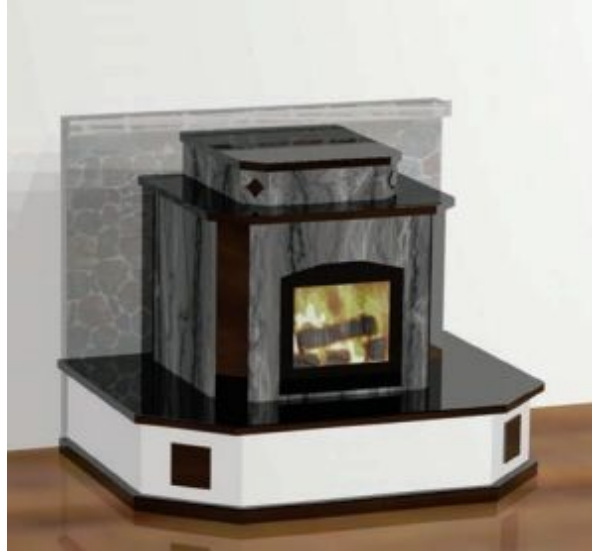
FIGURE 8.10. The final design. The owner, however, rejected the use of white stucco in favor of soapstone for the bench supports.
