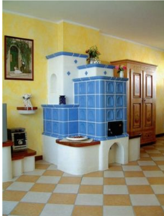
FIGURE 6.42. A real kachelofen ; it's a masonry heater built with structural tiles. Photo courtesy of Biofire, Inc.
