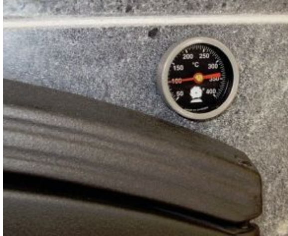
FIGURE 11.17. A long-stemmed thermometer registers the temperature of the masonry above the oven. This one reads in degrees Celsius.
