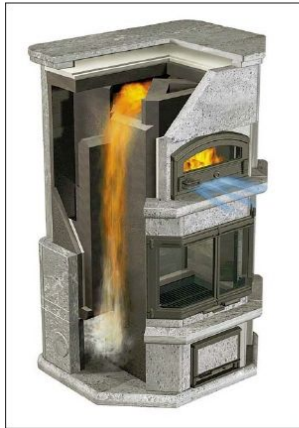
FIGURE 11.16. A cutaway view shows the smoke path from a black oven in a Finnish contraflow design. The exhaust goes briefly up, then down both sides before exiting into a chimney connector. Illustration courtesy of Tulikivi Corporation.
