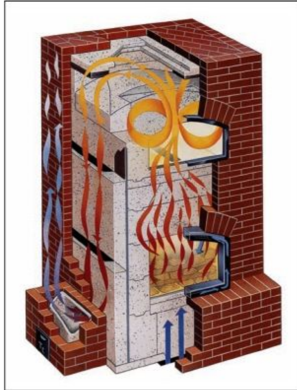
FIGURE 8.57. A cutaway view of the Temp-Cast heater shows the large tongue-and-groove blocks of cast refractory components in light gray. Illustration courtesy of Temp-Cast Enviroheat.
