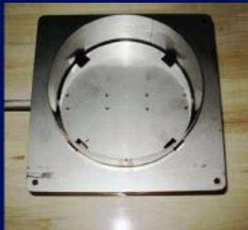
FIGURE 7.14. The damper in the closed position. Slots and a loose fit make this a 95 percent closure damper.
